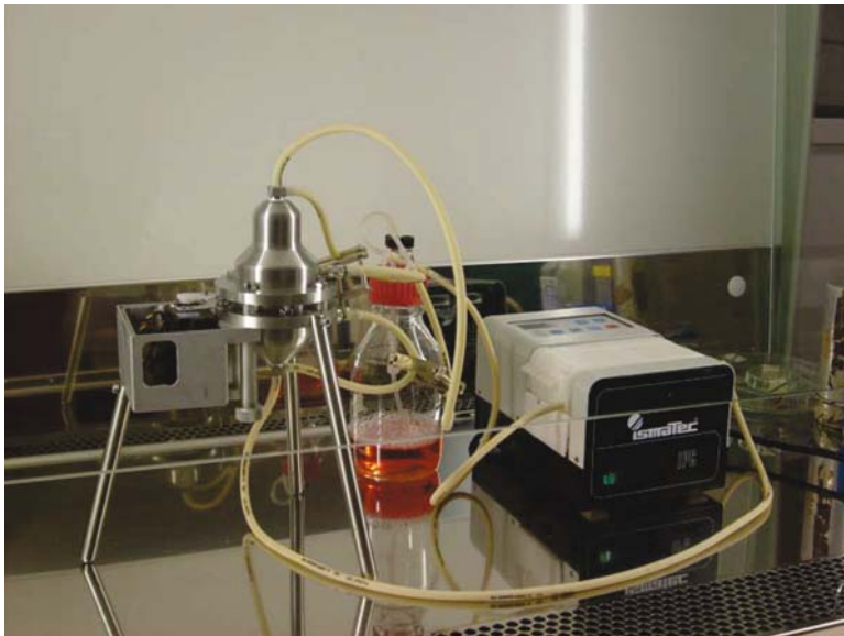
Fig. 6 Prototype of a new laminar flow perfusion bioreactor during its testing phase
