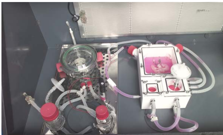
Fig. 3 Bioreactor for the generation of vascularised tissue with an arterial inflow and a venous reflux system. In the bioreactor a scaffold for the in vitro generation of vascularised liver tissue is inserted and connected to an arterial supply to provide fresh nutrients to the culture medium. The metabolites are then removed with the pulsatile flowing medium through the venous reflux system into the smaller chamber. The small chamber and the larger chamber are connected, providing a closed circulation. Using this bioreactor we are able to simulate the natural environment of the body, from blood pressure to temperature and control and regulate the culture conditions during the whole culture period
