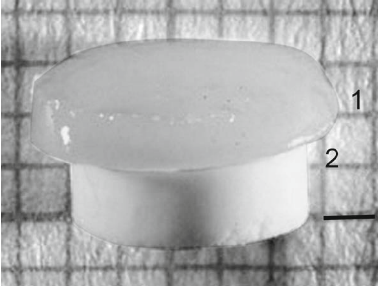
Fig. 2 Cartilage carrier construct from porcine chondrocytes, side view of a cartilage-carrier construct (1: newly formed cartilage by free swelling, 2: solid calcium phosphate carrier, scale 1 mm)
