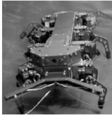
Figure 6.38 The octopod robot developed by Applied AI Systems Inc. was used for various evolutionary projects described in the text.
