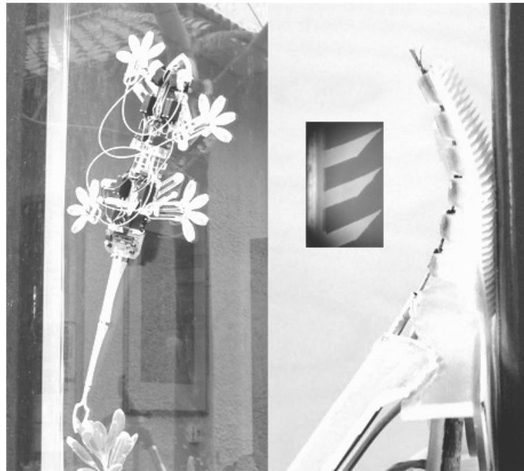
Figure 6.20 Stickybot with detail of the retractable footpads and of the anisotropic artificial setae. Images courtesy of Mark R. Cutkosky, Stanford University, Stanford, CA.
