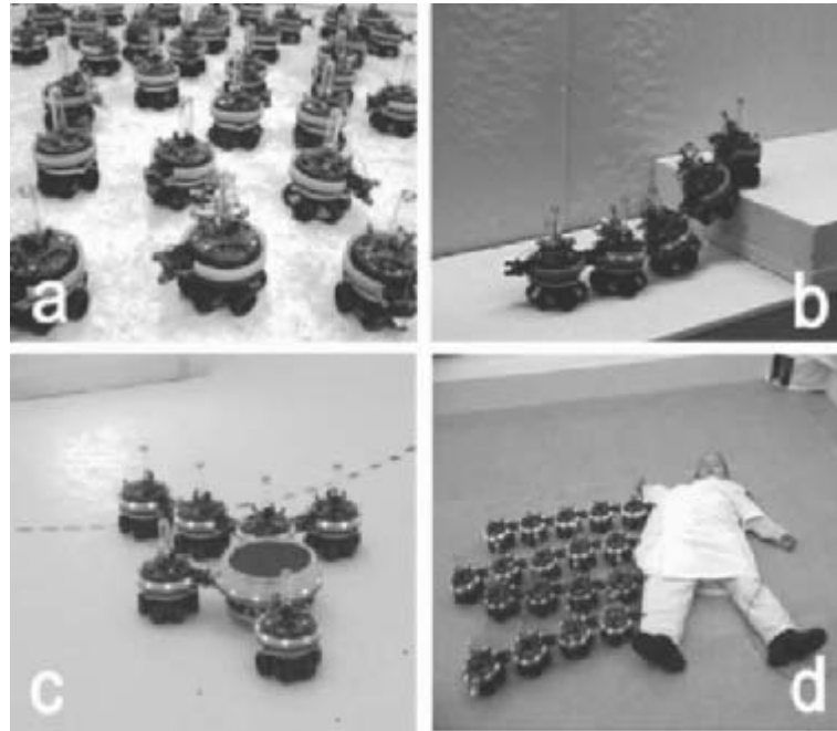
Figure 7.17 Swarm-bots are composed of several s-bot units that can operate in isolation or in physically connected assemblies (Mondada et al. 2004). a , A group of s-bots are deployed for coordinated search. b , A Swarm-bot of five s-bots is passing over a step. c , A Swarm-bot of five s-bots transports a heavy object towards a target region. d , A Swarm-bot of 18 s-bots pulls a child to a safe location.
