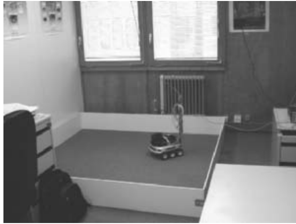
Figure 6.47 A mobile robot with a pan-tilt camera is asked to move within the walled arena in the office environment.
