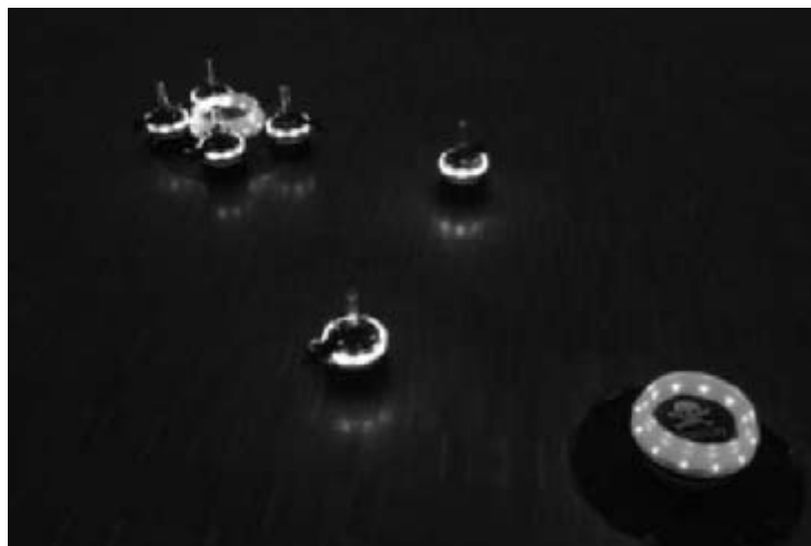
Figure 7.35 A team of s-bots engaged in cooperative communication (Floreano et al. 2007). A group of four s-bots feed on the food objects while they are lighted up in blue color. Two s-bots in white color are attracted by the blue signal and move away from the poison object.
