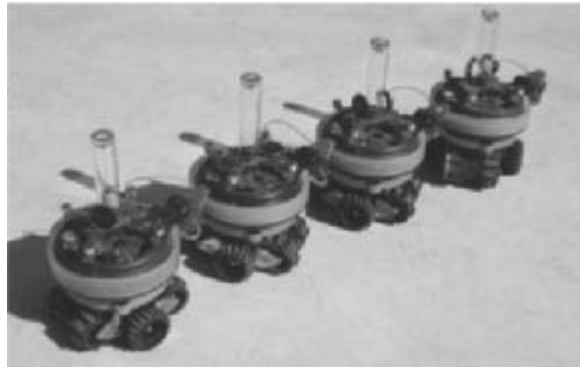
Figure 7.34 A Swarm-bot composed of four interconnected s-bots in chain formation.
