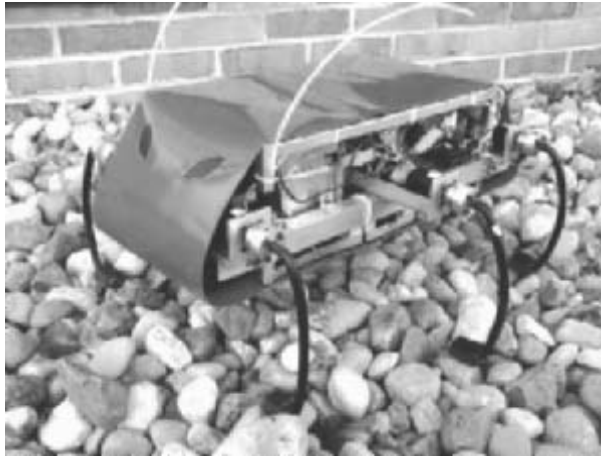
Figure 6.16 RHex is a simple hexapod robot capable of tripod gait and navigation on rough terrains ( www.rhex.org ).
