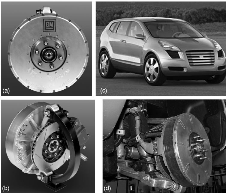
Fig. 9.15. GM's Sequel fuel cell concept electric vehicle: (a) Front view of the AFPM wheel motor, (b) Back view of the AFPM wheel motor, (c) Sequel FCEV, (d) Rear AFPM wheel motor with electromechanical brake, rear steering actuator and integrated controlled damper. Courtesy of General Motors Corporation , U.S.A.
