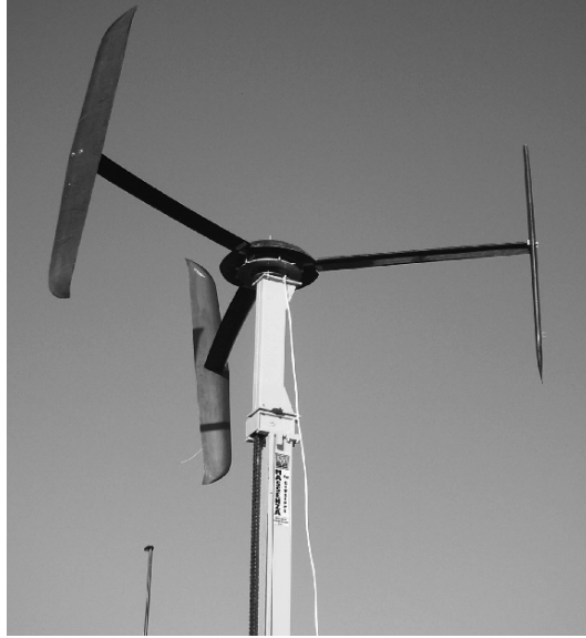
Fig. 9.7. Generator integrated with a vertical axis wind turbine. Courtesy of Durham University and Carbon Concepts , UK.
