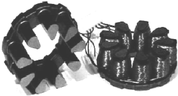
Fig. 2.12. Three-phase, nine-coil stator of a single-sided AFPM brushless machine with salient-pole stator. Photo-courtesy of Mii Technologies , Lebanon, NH, U.S.A.
