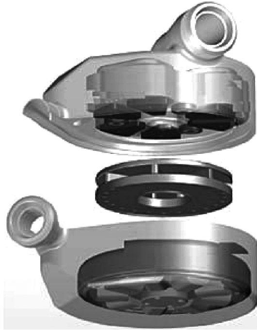
Fig. 9.34. Exploded view of DuraHeart R centrifugal rotary pump. Courtesy of Terumo Corporation , Tokyo, Japan.
