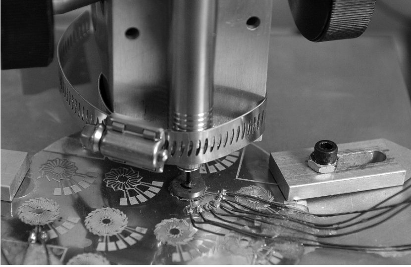
Fig. 5.3. Experimental tests on AFPM microgenerators by spinning a small magnet with the aid of air-powered drill above a mesh of coils fabricated on a chip. Photo courtesy of Georgia Institute of Technology, Atlanta, GA, U.S.A.
