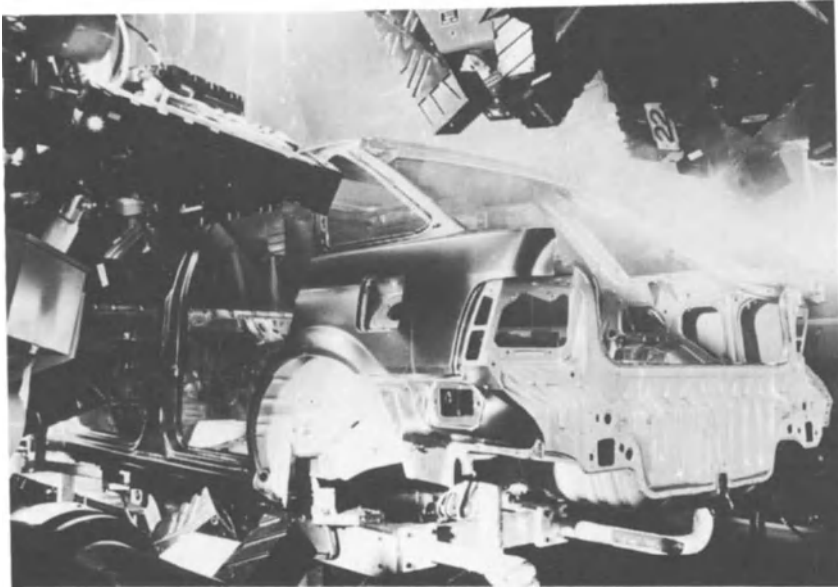
Figure 14.6 Rover 200/400 series body gauging station.
