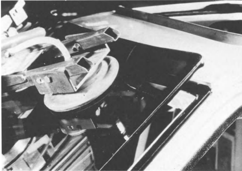
Figure 14.10 Close-up view of robotic fitment of front glass to car.
