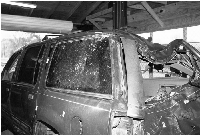
FIGURE 15.14 Rear lift gate damage from tree impact.
