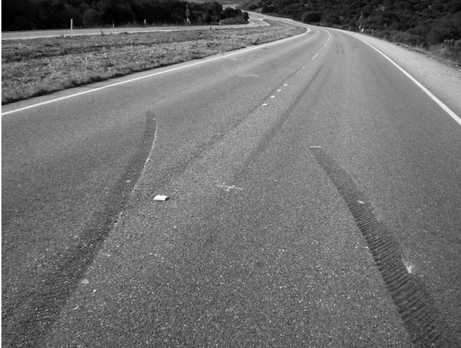
FIGURE 15.1 Cessation of tire marks at roll initiation.
