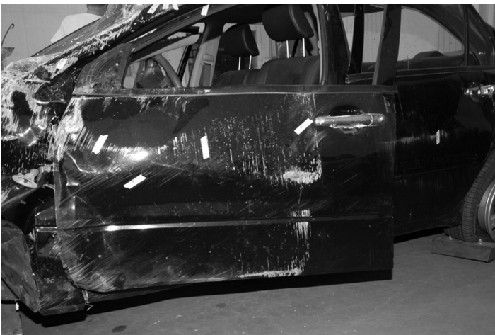
FIGURE 15.22 Effects of pavement edge on vehicle.
