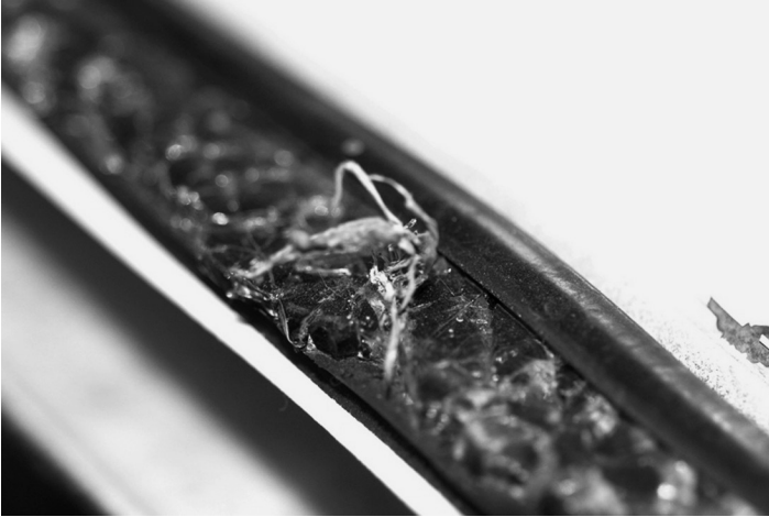
FIGURE 15.12 Wood fibers trapped in weather seal.
