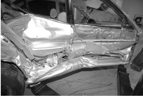
FIGURE 22.1 Crush profiles marked with inch tape.
