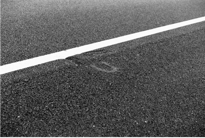
FIGURE 15.19 Crescent mark visible at scene inspection.
