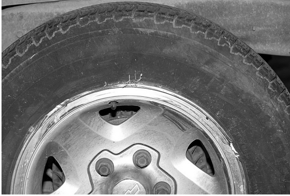
FIGURE 15.21 Plant materials in wheel rim.
