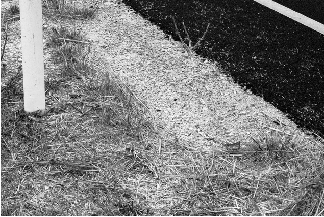
FIGURE 15.26 Glass deposit long post-accident.
