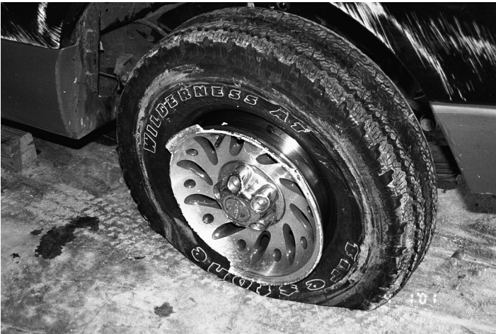
FIGURE 15.16 Fractured wheel with two impacts.
