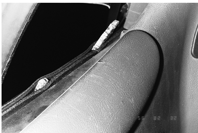
FIGURE 15.25 Ejection portal evidence.
