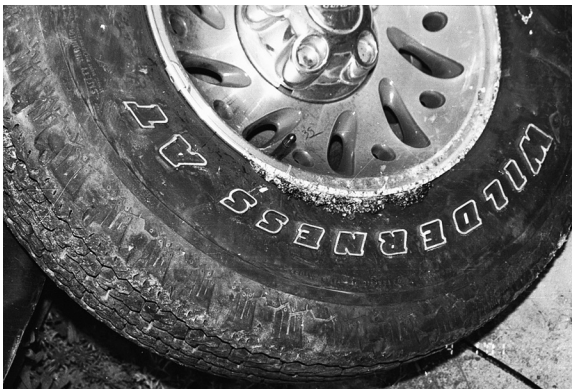
FIGURE 15.20 Asphalt deposits in wheel rim.
