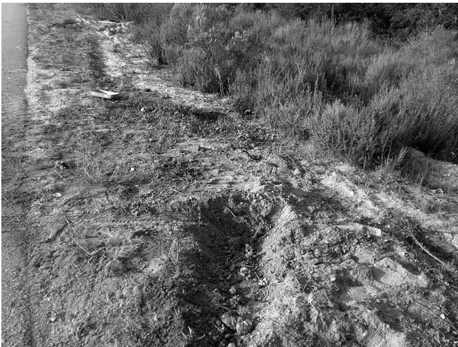
FIGURE 15.2 End of furrow at roll initiation.
