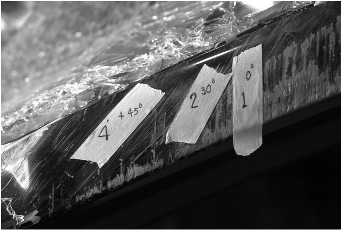
FIGURE 15.7 Example of scratch pattern demarcation.
