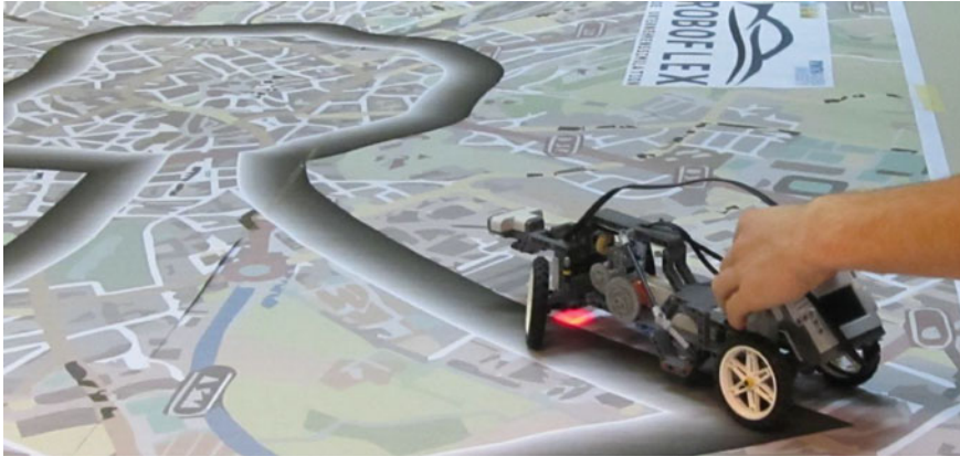
Figure 4 Autonomously driving Lego Mindstorms NXT robot in ROBOFLEX
