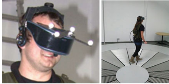
Figure 3 Head mounted display and omnidirectional floor of the virtual theatre
