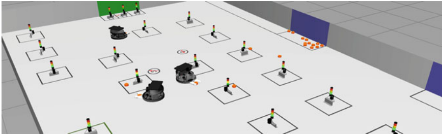
Figure 8 The simulation of the LLSF in Gazebo. The circles above the robots indicate their localization and robot number
