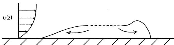
Fig. 5. Profile-view sketch of a heavy fluid collapsing into a shear flow.
