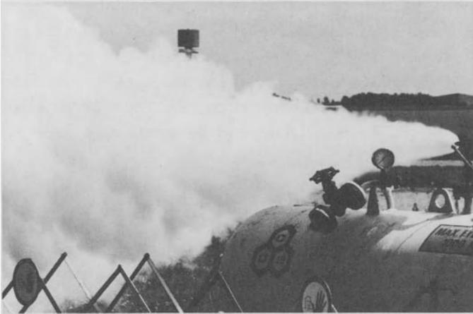
Fig. 2. The close-up shows the 1/2" release pipe and the rapid expansion of the jet diameter in the outflow region. The photo also gives an impression of the complete obscuration of the jet due to the CO<sub>2</sub>-aerosol.
