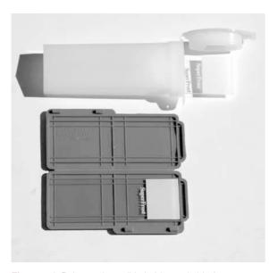
**Figure 1.2** Polypropylene slide holders suitable for transporting blood smears.
