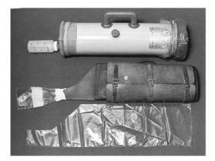
**Figure 7.32** Assembled CSU model (top) and Missouri Artificial Vagina (middle) with plastic disposable liner (bottom).
