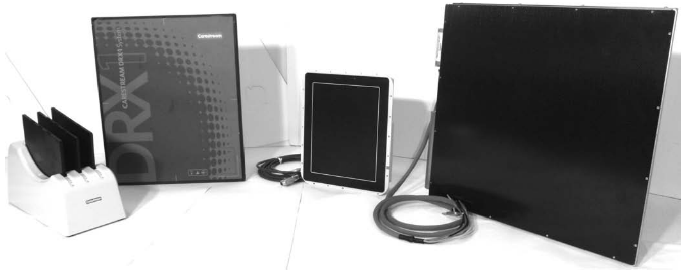
FIGURE 10.3 Examples of the variety of flat-panel detectors. From the right the detectors are a projection radiography detector (Trixel 4600), a small format fluoroscopic detector (Varian Paxscan 2520), and one of the new film-cassette-sized, wireless, battery-powered detectors recently introduced into the market (Carestream DRX-1 shown with battery charger).
