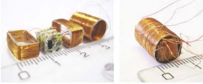
Figure 8. (a) Three orthogonal coils and receiver electronics integrated on a stack of thick-film substrates. (b) Electronics and coils assembled for integration in capsule.
