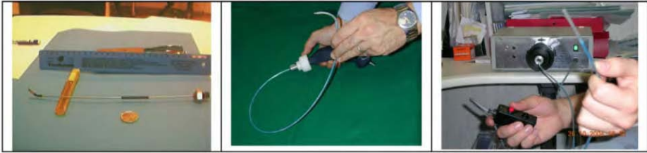
Figure 4. IVP1 steering: the movable tip (l), steering with a handle (m), motor driven system (r).
