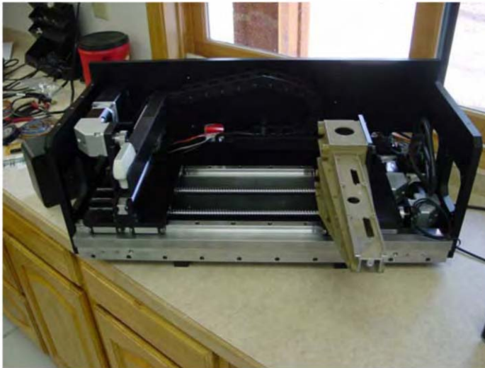
Figure 3. Assembly of lower gantry of FFD MUS showing the fusion of X-ray detector and ultrasound transducer.
