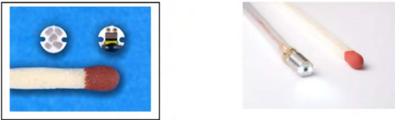
Figure 3. Ceramic board with IVP1 image sensor and pad connectors (left), IVP1 videoprobe head with optics and illumination (right).
