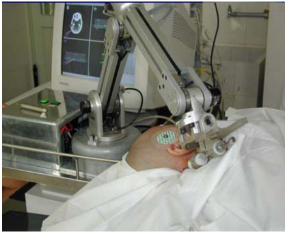
Fig. 3. The biopsy procedure for brain stem lesions. When mechanical arm arrives at the accuracy position according to the surgical plan, it guides puncture needle to arrive at target followed by biopsy on the operation platform.
