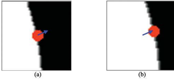
Fig. 2. The method to find the corresponding point. The white regions stand for the foreground, while the black regions mean the background. The red point in (a) is an original point on the edge of I_i , and its corresponding point on the edge of I_j is the red point in (b), which is found along the normal direction denoted as blue arrow.
