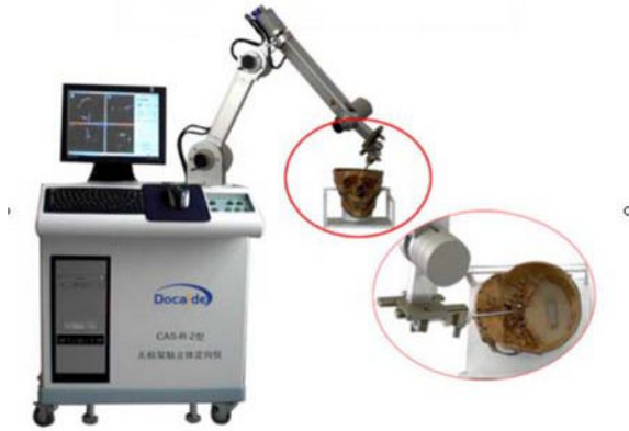
Fig. 1. The CAS-R-2 robot system. The instrument roughly consists of computer, software and mechanical arm with five-degree freedom.
