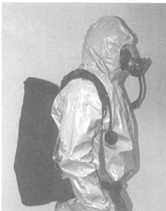
Figure 22.4 Responder wearing a level B ensemble consisting of a self-contained breathing apparatus and a splash-protective non-woven polymer coverall. Photo courtesy of the University of Missouri Fire and Rescue Training Institute.
