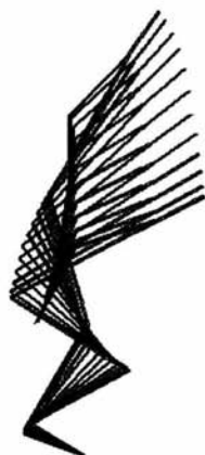
Fig. 5.67. Kinematic scheme of the 7-element model motion (raising up from a semi-squatting position, pre-set kinematics).
