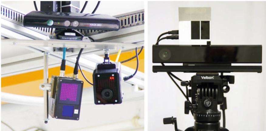
**Fig. 1** *Left* Sensor node with Kinect (*top*), ToF camera (*bottom center*); the optical tracking (*bottom right*) was not used for this work. *Right* Argos P100 3D mounted on top of Kinect II
