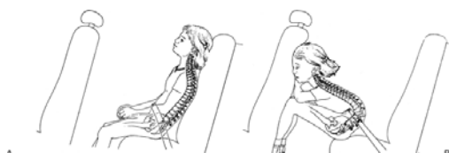
FIGURE 5. A: A child with typical slouched posture; note poorly developed anterosuperior iliac spine. B: Frontal collision; lap belt slips over iliac crests to focus bending force in the midlumbar region.
