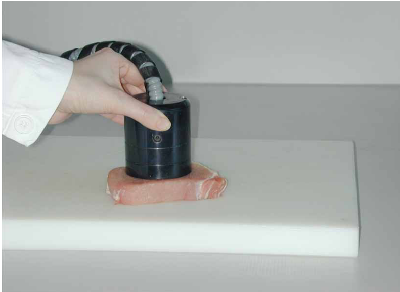
Figure 5. Colorimetry of fresh meat cut surface after 1-2 hours of exposure to air.
