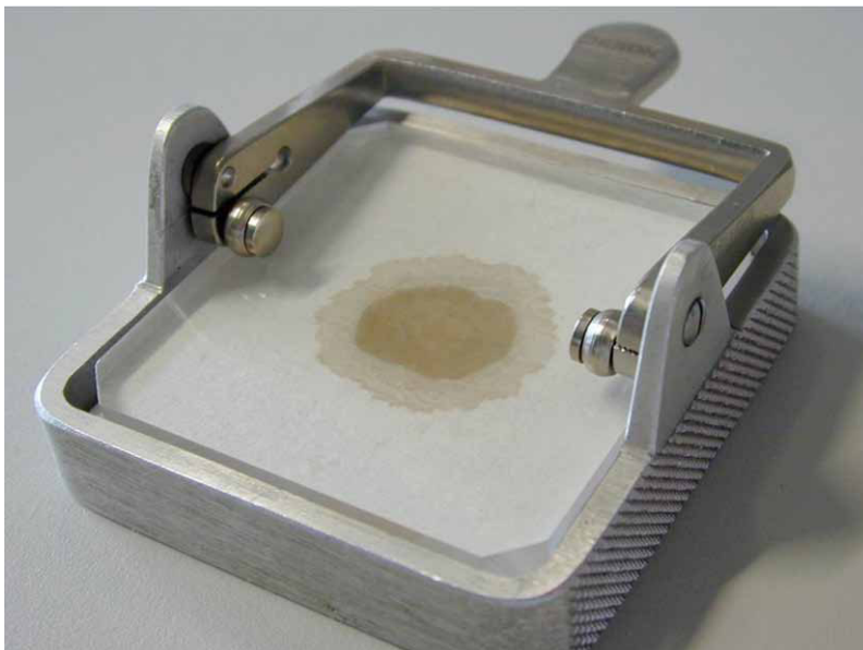
Figure 1. Measurement of the water holding capacity of fresh meat by the press-method (Grau and Hamm, 1953).
