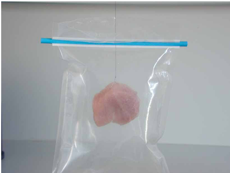
Figure 2. Assessment of water holding capacity by measuring weight loss over time in suspended fresh meat samples.
