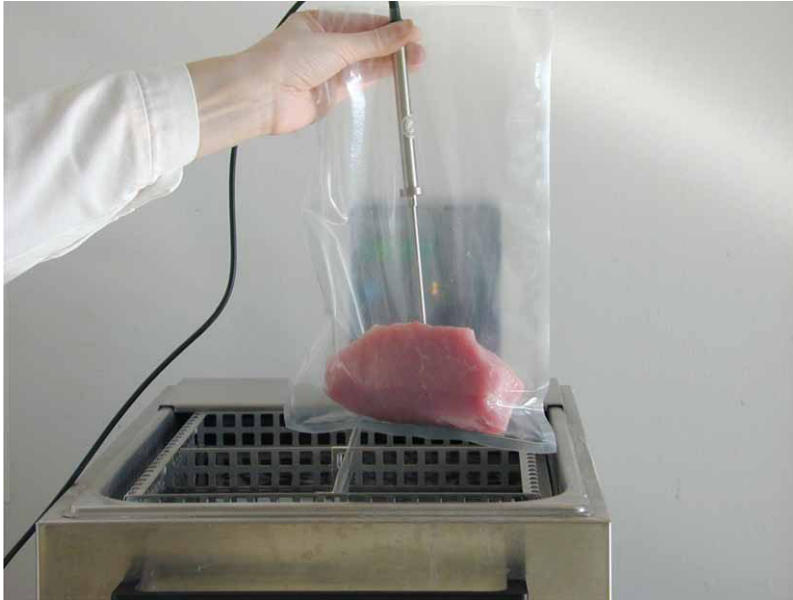
Figure 3. Assessment of cooking loss by measuring weight differences before and after heating in a water bath.
