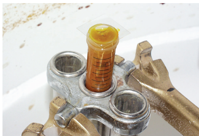
Figure 15-11. Centrifuge with free swinging buckets showing a coverslip in place before centrifugation.
