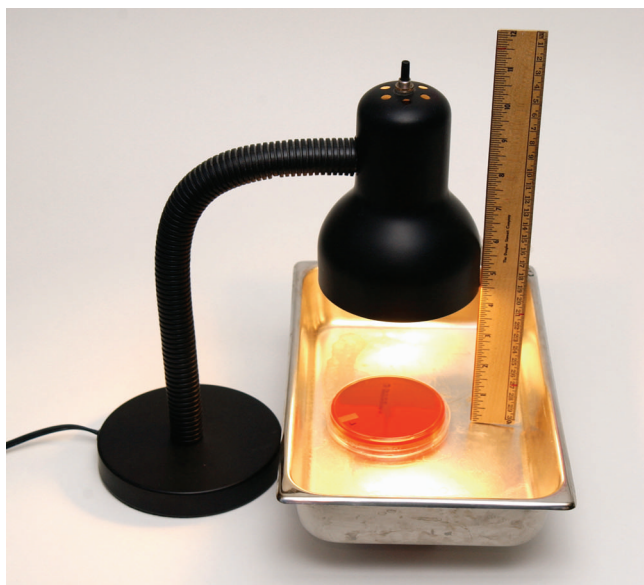
Figure 48-4. Incubation of an inoculated blood agar plate with urine under a 60-watt incandescent light bulb. Surface temperature of the blood agar plate is 37° C.
