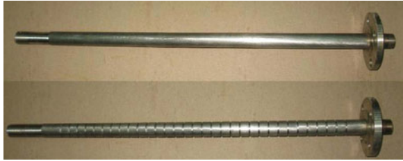
Fig. 28.2 Photograph of transversally grooved tube and smooth tube
