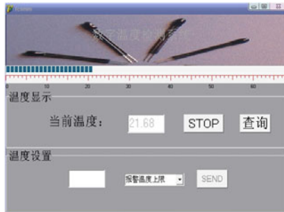
Fig. 4. Remote monitoring software interface
