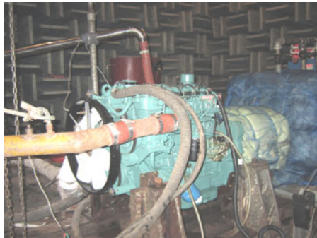
Fig. 1. Diesel engine and dynamometer installation diagram
