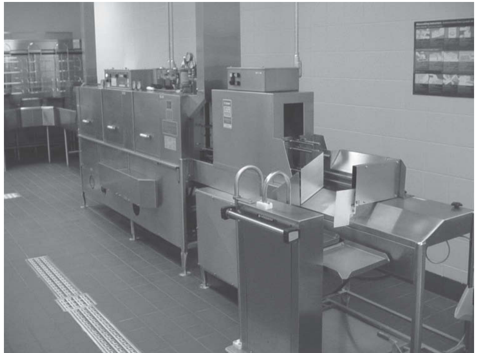
Figure B-20 Machine designed especially for washing trays.
