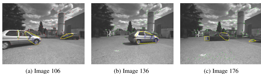
Fig. 7. Algorithm results for occlusion objects. Gray car is detected by two different regions then it is totally detected several images later. A second car that crosses the scene is detected before and after its total occlusion.
