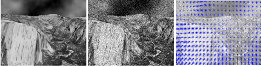
Fig. 5. Left: Yosemite sequence. Centre: We added Gaussian noise with standard deviation \sigma = 40 . Right: The shown high quality optical flow field is obtained by the control based optical flow approach (4) - (5) (parameters: \alpha = 0.05 and \beta = 0.000003 ).
