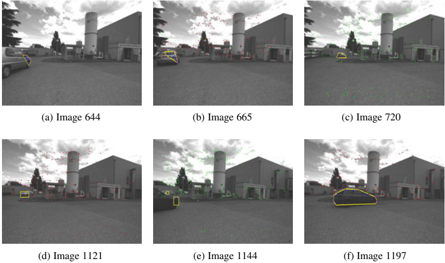
Fig. 9. Experimental results in outdoor environment. First row shows moving object detection and tracking for a car that moves in the same sense of the robot, furthermore it does not cross the field of view of the robot. On the second row: moving object detection before the occlusion is successfully handle by our proposed method.
