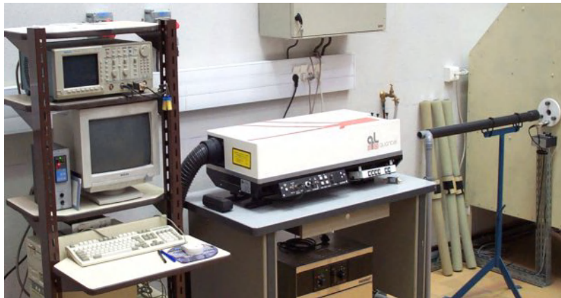
Figure 13.3. View of an experimental setup (digital oscilloscope and signal-processing computer on the left, laser generator at the center and measurement cell on the right)
