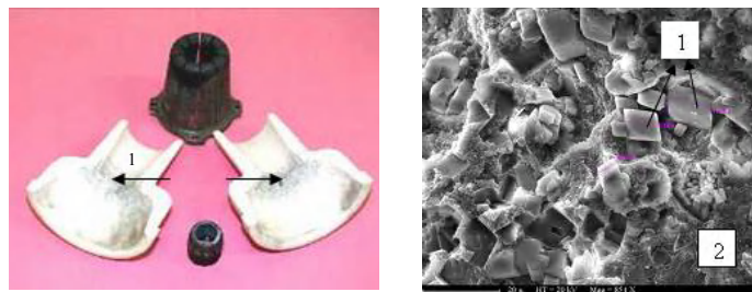
Figure 24.2. (a) Nozzle and contact of the equipment (1: ablation zone of the nozzle) (b) Microstructure of the nozzle (1: mineral charge – 2: PTFE)
