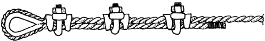
Figure 13-11. Correct Placement of Cable Clamps.
