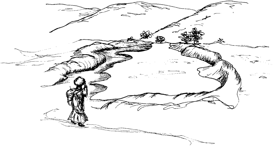
Figure 17-2. Small Check Dams Were Historically Constructed in India to Slow the Movement of Surface Runoff and Thus Enhance Groundwater Recharge.
