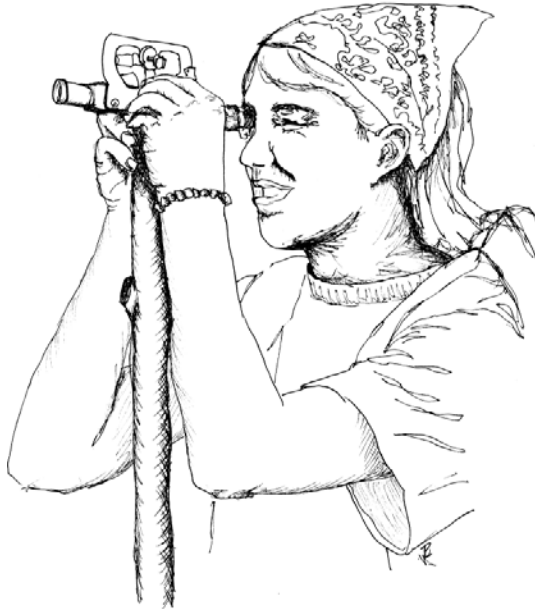
Figure 5-3. Measuring the Angle of Inclination with an Abney Level.
