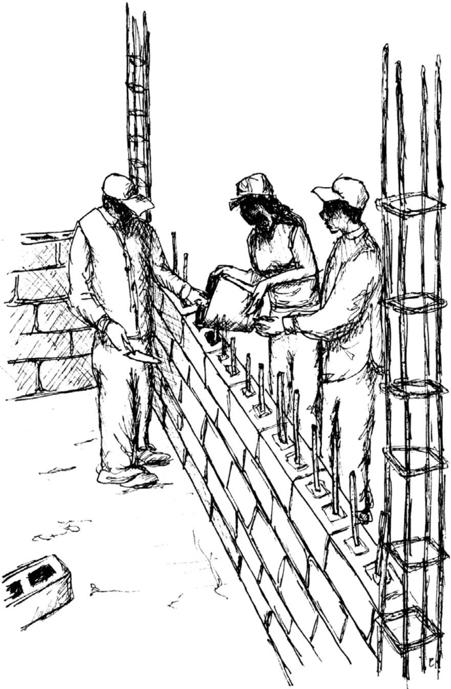
Figure 7-24. Concrete Block Installed over Vertical Rebar. Workers Are Filling Hollow Cores with Grout to Create a Reinforced Concrete Block Wall.
