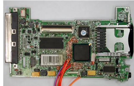
Figure 6.3 Sensor mounting for product test. (a) Strain gauge and accelerometer mounted on board assembly. (b) Strain gauges around package, with lead wires connected to gauges.
