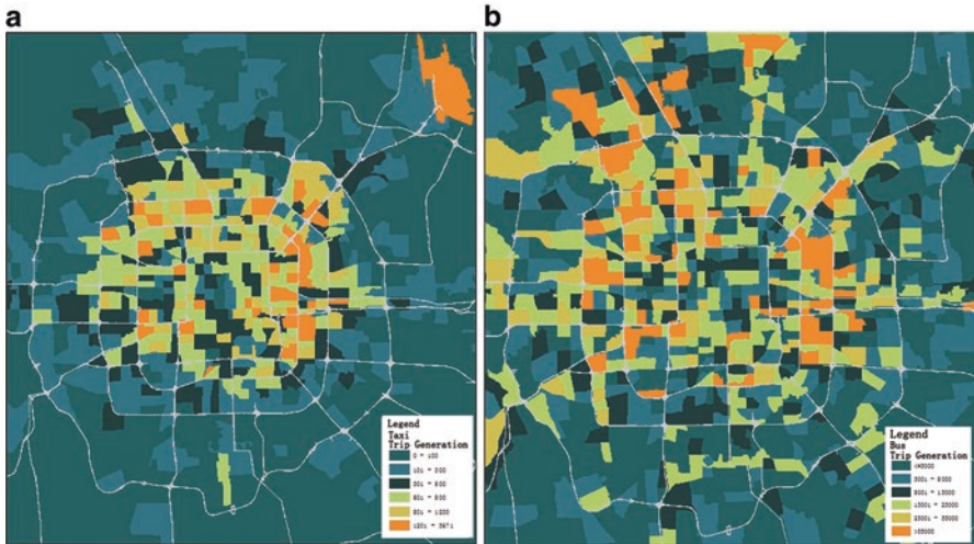
Fig. 12.9 Relative popularity of space unit for different transport modes. *Metro stations and suburban bus stations excluded. (a) Taxi trip generation. (b) Bus trip generation
