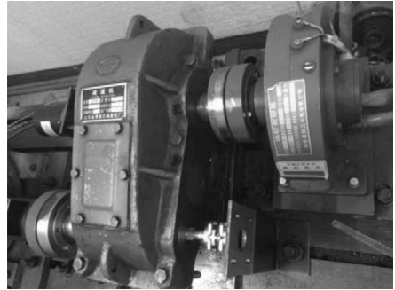
Figure 3. Picture of the single-stage gearbox vibration test.
