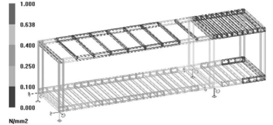
Figure 7. Distribution of stress ratio in the model of the redesigned unit.
