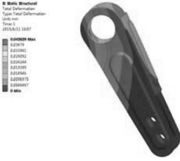
Figure 3. Graph of arm deformation.
