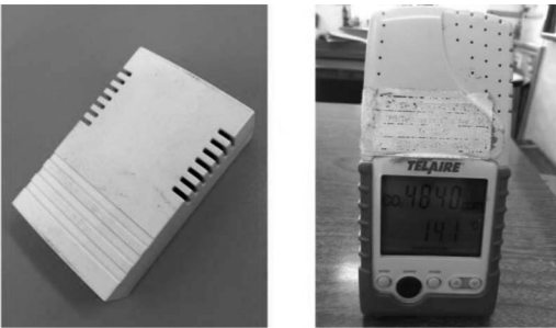
Figure 3. RR002 temperature/RH logger and hand-held AZ7752 temperature/CO 2 tester.
