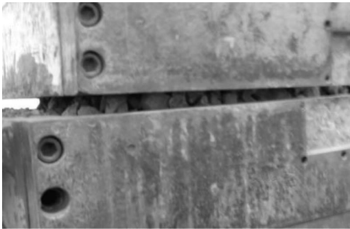
Figure 6. Opened shear box.
