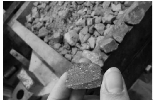
Figure 8. Broken particles by shear.
