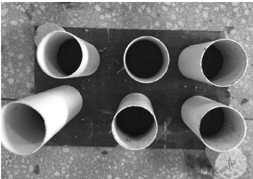
Figure 1. Picture showing specimens for shear tests.
