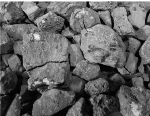
Figure 12. Edges and corners smashed and long flat shape particles breaking off.
