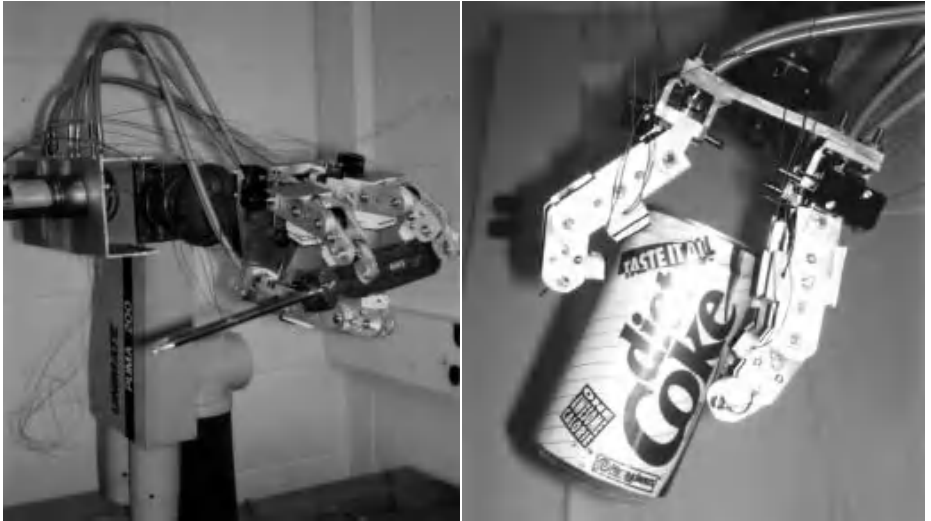
Fig. 5. The Graspar Robot Hand. The left side of the figure shows Graspar mounted on a Puma 200 holding a screwdriver in a fingertip grasp. The right side shows a close up of the hand holding a soda can in an enclosing grasp from the top of the can.
