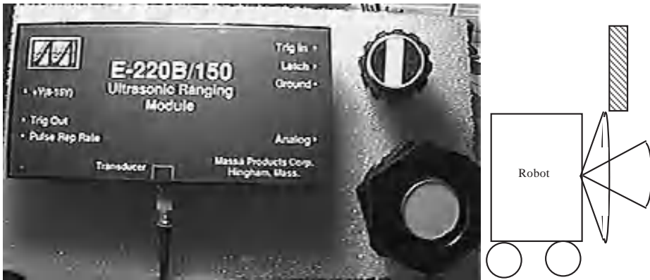
Fig. 6. New directional acoustic transducer produced by Massa Products Corp., Hingham, MA. The left shows the electronic control box for properly amplifying the return signal to be in the appropriate range for analog to digital conversion. The bottom right shows a standard Massa acoustic transducer in a mountable casing. The top right is the directional transducer. Notice that the ceramic surface of this transducer is masked to be linear rather than circular. The drawing on the right illustrates this transducer’s usefulness for detecting overhanging obstacles compared to a standard conic sonar.
