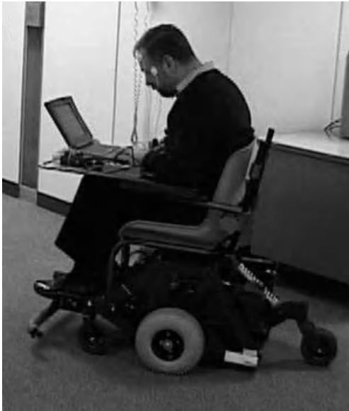
Fig. 4. The robotic wheelchair system being driven using EagleEyes, an eye tracking system.
