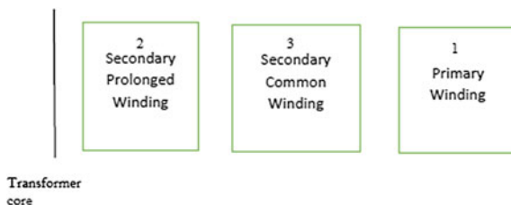
Fig. 5 Single-phase model wiring arrangement
