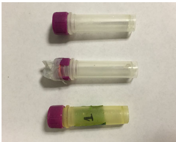
Fig. 3 Differences in the same lot of polypropylene sample vials after neutron activation of the Ho-MSN powders. ( Left vial ) 8 h in neutron flux caused extreme flimsiness in the vial and discoloration. ( Middle vial ) The cap was cracked while attempting to open it. ( Right vial ) Vial was carefully opened and did not present any noticeable breakage
