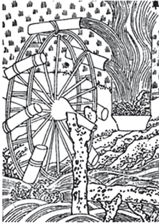
Fig. 2.8 Bamboo water wheel (From the Nong Shu [86,141])
