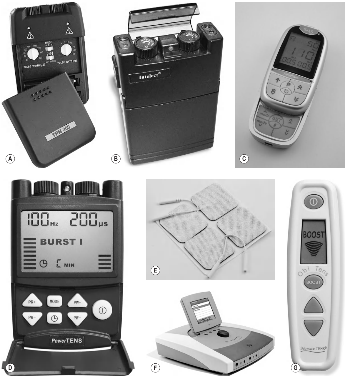
Figure 19.3 TENS machines and electrodes: (a) analogue TENS (Body Clock); (b) analogue TENS (Chatanooga); (c) digital TENS (TensCare); (d) digital TENS (Natures Gate); (e) self-adhesive electrodes (TensCare); (f) multimodal stimulator including TENS (Enraf); (g) obstetric/maternity TENS (Body Clock).
