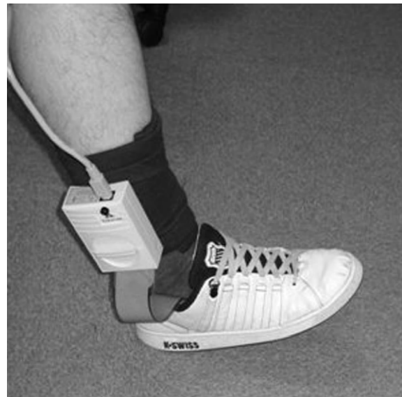
Figure 15.39 In-shoe Pressure Measuring System (F-Scan, Tekscan Inc., South Boston, MA, USA).
