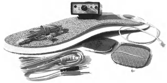
Figure 19.16 Odstock dropped foot stimulator. Salisbury ODFS111 stimulator, innersoles, footswitch, electrode pads and leads. The stimulator is a single channel device designed primarily for gait assistance. (Courtesy of the Department of Clinical Science and Engineering, Salisbury District Hospital, UK.)
