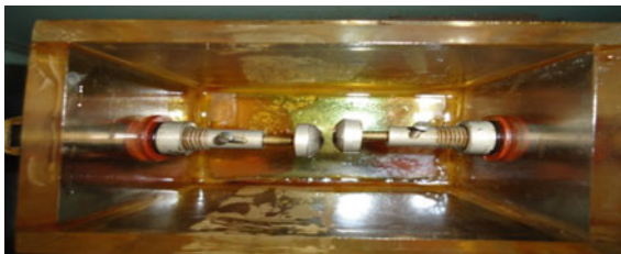
Fig. 1 Breakdown voltage measurement test cell with electrodes
