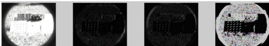
Fig. 30.8 Results of the 12 am image processing. First one is the original picture, second and third are the polarization intensity pictures, and the last is DoP picture
