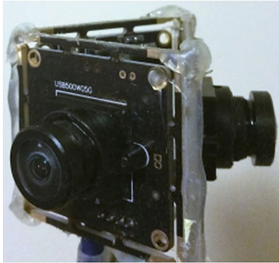
Fig. 1 The proposed 3-camera rig for generation of 360° panoramic videos
