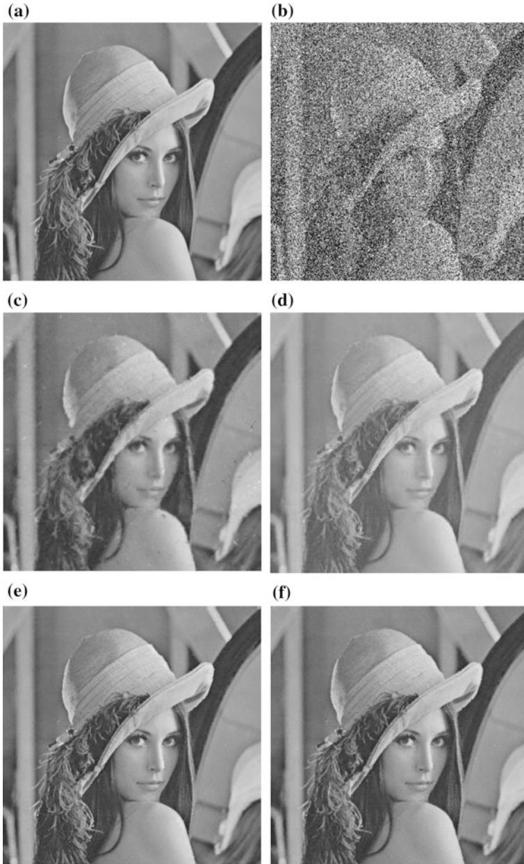
Fig. 1 Output results for Lena image with 50% noise density. a Original image; b noisy image; c output image of the DWM filter; d output image of the modified DWM filter; e output image of the LGII method; f output image of the proposed method
