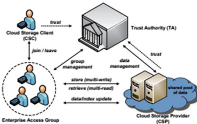
Fig. 1 Enterprise cloud storage access model
