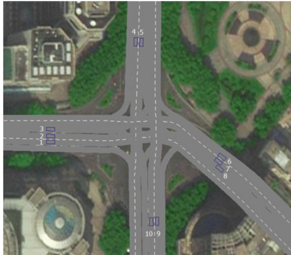
Fig. 2 Position of detectors of the intersection
