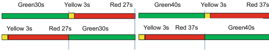
Fig. 3 Intersection signal timing diagram at present. a Scheme 1. b Scheme 2
