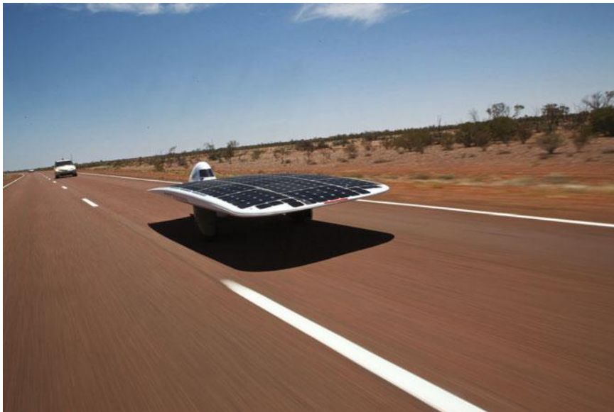
Figure 3.3 As well as being used in rooftop and grid-connected applications, 22 per cent efficient monocrystalline PV cells were used by Sunswift IV, the winning silicon solar car at the 2009 World Solar Challenge held in Australia
