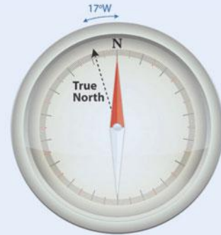
Figure 2.24 In Seattle magnetic north is always 17^\circ east of true north
