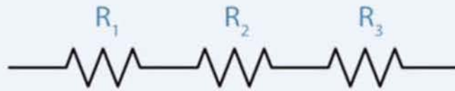
Figure 4.1 Resistors connected in series
