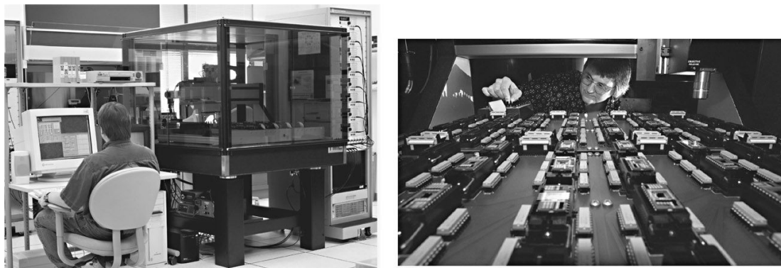
FIGURE 10.36 SHiMMeR system with multiple packaged part, computer control, data acquisition, vibration isolation, humidity enclosure, and video microscope. (Courtesy of Sandia National Laboratories, Radiation and Reliability Physics Department.)
