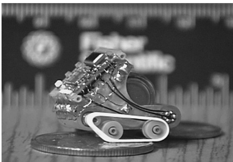
FIGURE 1.5 A small robot with a sensor, locomotion, control circuitry, and self power. (Courtesy of Sandia National Laboratories.)
