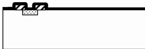
(b) Deposit and pattern metal contacts, passivate with silicon nitride
