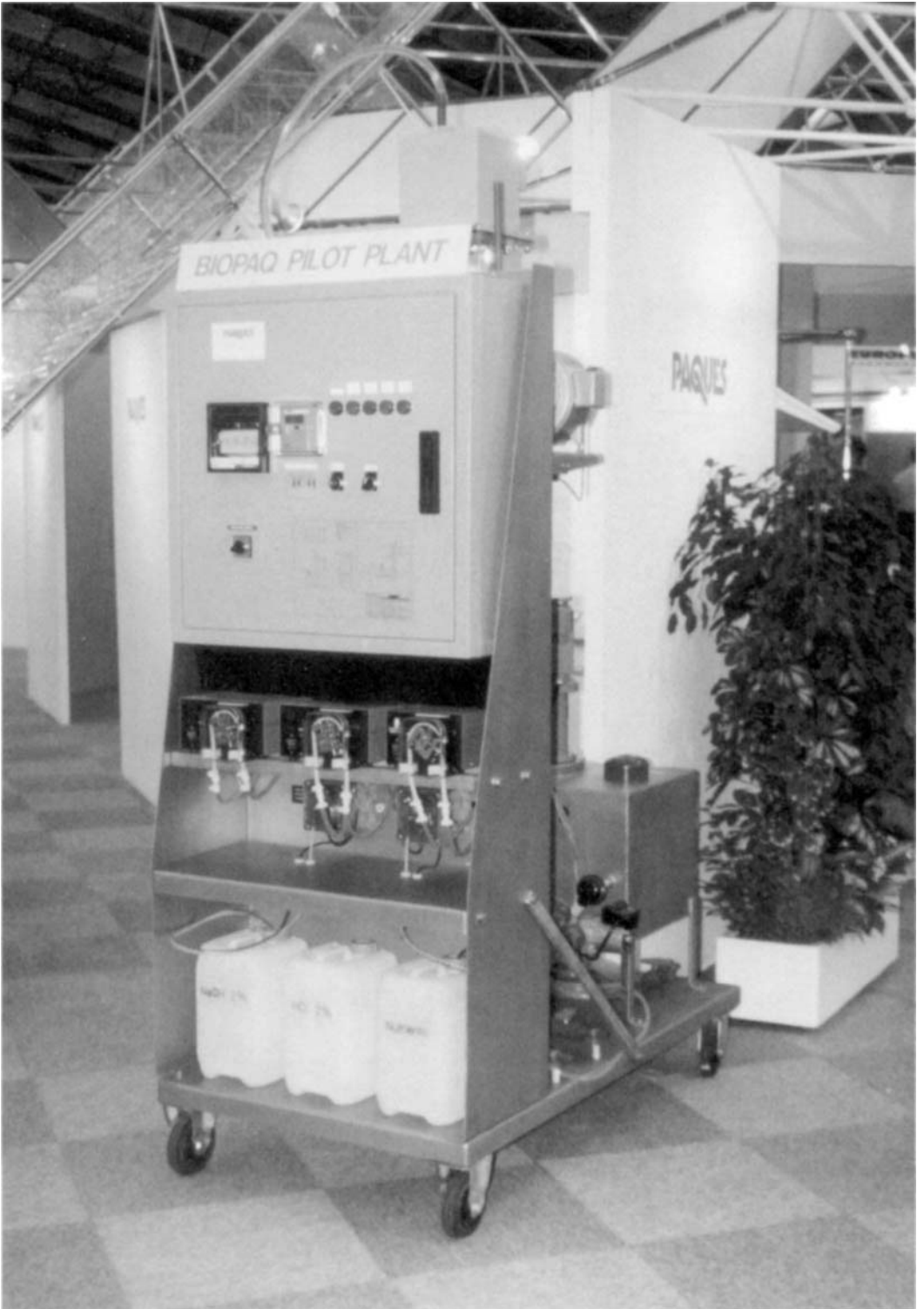
Figure 1-4 Photograph of a pilot-scale wastewater treatment system.
