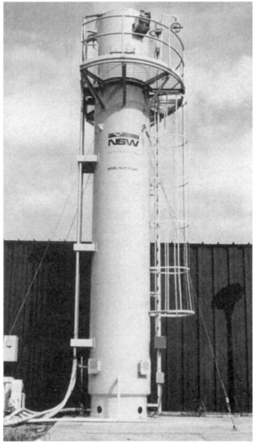
Figure 7-47 Aerobic fixed-film systems: (a) rotating biological contactor (courtesy of U.S. Filter/Envirex); (b) trickling filter (courtesy of NSW Corporation); (c) fluidized bed (courtesy of NSW Corporation).
