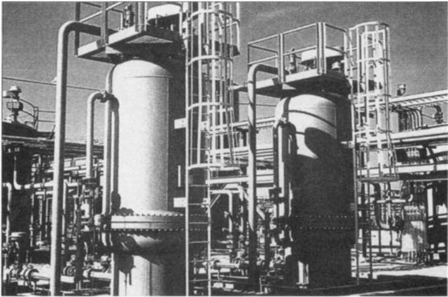
Figure 7-78 Pressure and vacuum filters. (d, e) Courtesy of Eimco Process Equipment, a Baker Hughes Company.
