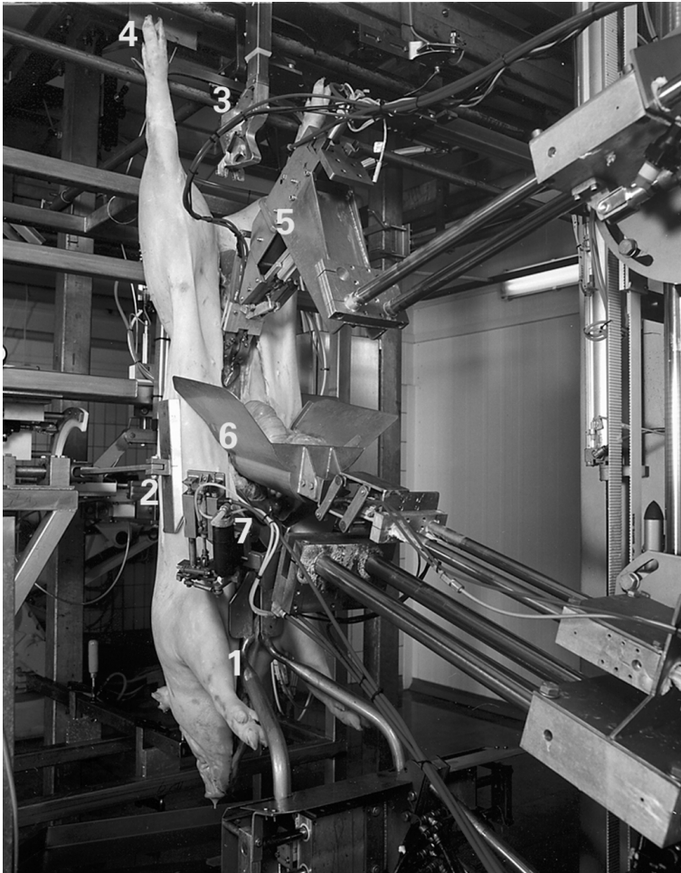
Fig. 14.1 Automatic evisceration system.
