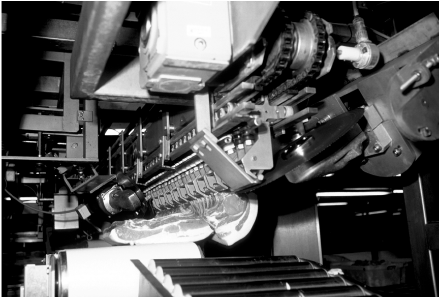
Fig. 14.2 Automated secondary processes: cutting of the middle.
