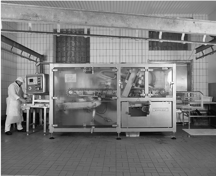
Fig. 14.3 Automated secondary processes: boning of the fore-end.
