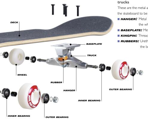
These are the metal axles to which the wheels are attached and that allow the skateboard to be turned while moving. Trucks are comprised of:
