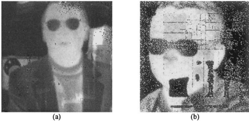
Fig. 20.15. Images from a: (a) GaInAs/InP QWIP and (b) InAs/GaSb type II superlattice (right) focal plane array camera operating in the 8\text{--}12 \mu\text{m} wavelength regime.
