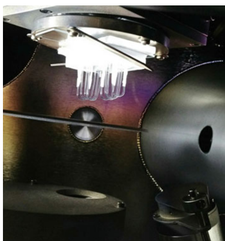
Fig. 7 Bare U-Shaped probes installed inside the sputtering chamber
