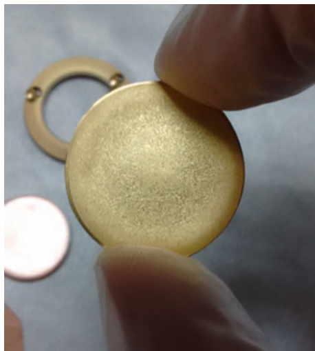
Fig. 6 Gold target used for U-Shaped probe coating by sputtering
