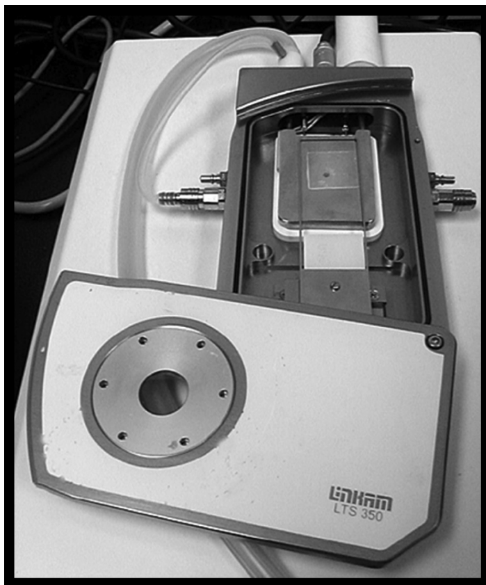
Figure 12 The Linkam LTS 350 microscope heating/cooling stage. The temperature of the sample is maintained by the use of a heating coil and liquid nitrogen, which are controlled by an external programmer and pump system (not shown).
