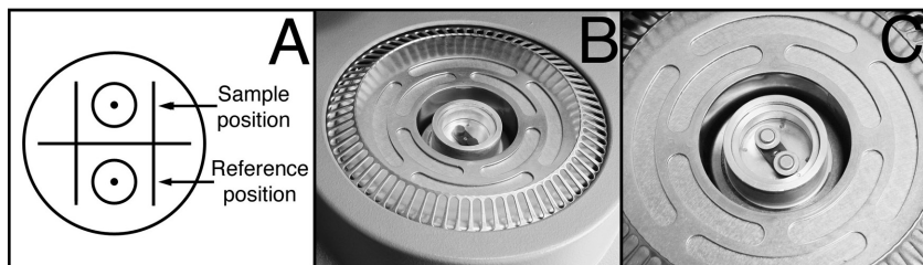
Figure 21 Positioning of reference and sample pans in a differential scanning calorimet (DSC) standard cell (A) (adapted from TA Instruments Advantage Manuals, TA Instruments, Mississauga, ON, Canada), view of an empty DSC cell (B), and view of a DSC with the sample and reference pans in position (C).
