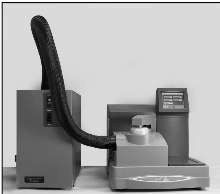
Figure 15 Differential Scanning Calorimeter (DSC) Q 1000 (TA Instruments, Mississauga, ON, Canada) used in the thermal analysis of edible fats and oils.
