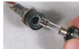
Panel fuse holder with glass fuse
