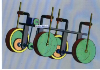
Fig. 5. The overall effect diagram of the new lunar rover based on planetary wheel mechanism
