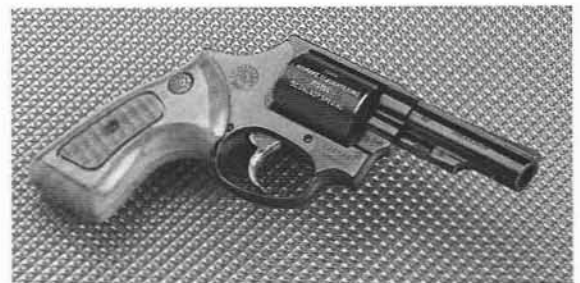
Fig. 8.3 Humane slaughtering pistol; single-shot/free bullet, .32 calibre. This instrument is not a stunner. (By kind permission of Messrs Accles and Shelvoke, Witton, Birmingham, UK)
