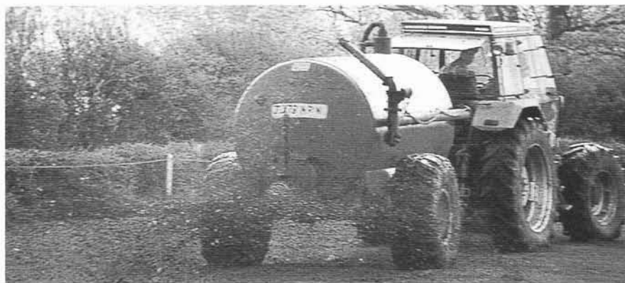
Fig. 7.6 Application of slurry by tanker spreader. (By courtesy of NW Water, UK)
