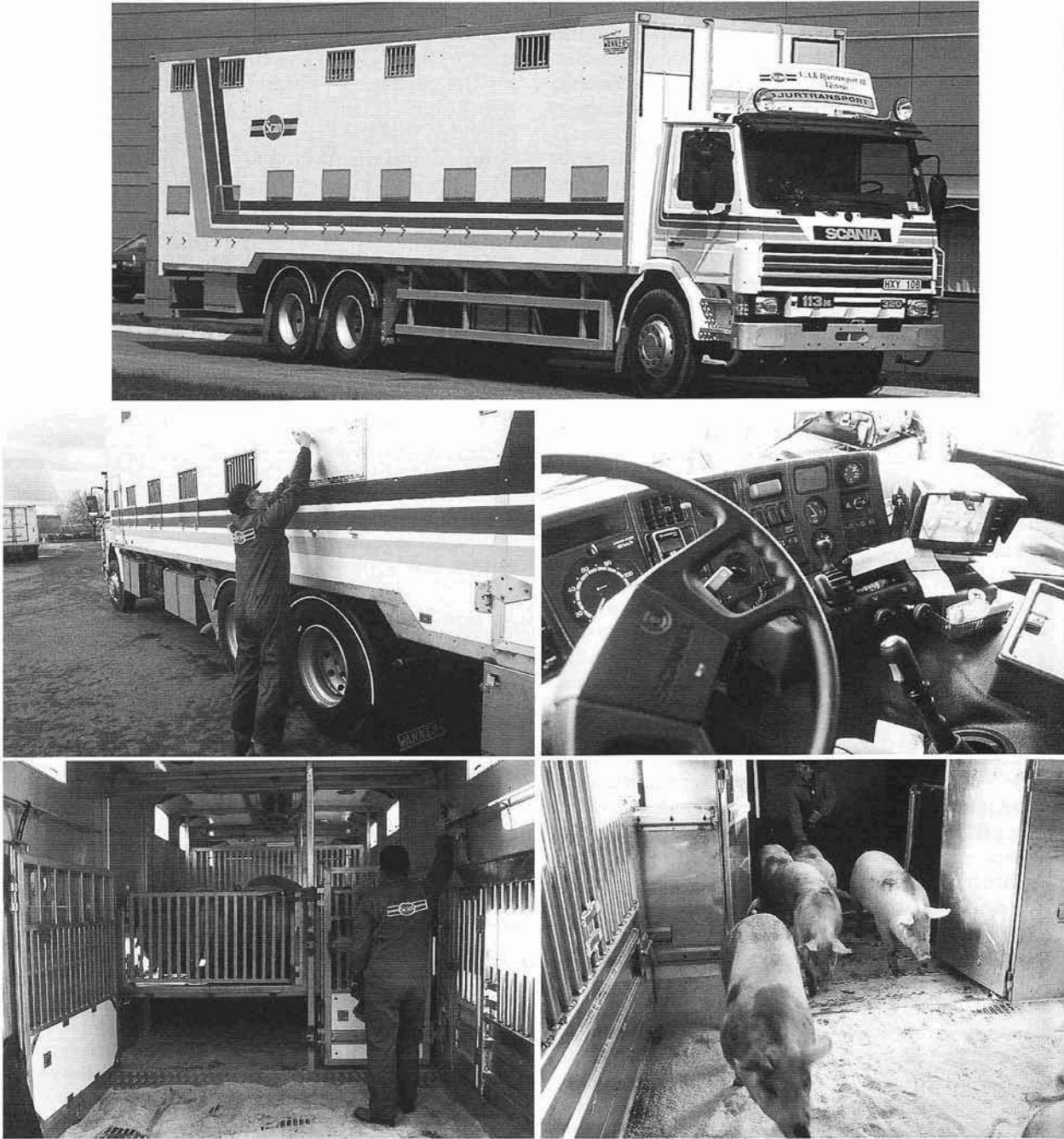
Fig. 7.9 Modern air-conditioned transport vehicle with separate designs for pigs and cattle. For pigs there are four sections at floor level and two at an upper level. Ventilation is achieved (air volume changed every minute) by four electric fans, 24 ventilation doors and three roof hatches. Ten recessed lamps provide interior lighting. A sprinkler system is available for use during higher environmental temperatures. Loading and unloading is hydraulically adjustable with side gates and interior doors. Two temperature measuring points are located in the vehicle and one in the cab where continuous visual monitoring of the animals during transit is possible. The vehicle is equipped with air suspension on all axles for maximum transport comfort. (By courtesy of Scan Farmek S-532 87, Skara, Sweden)
