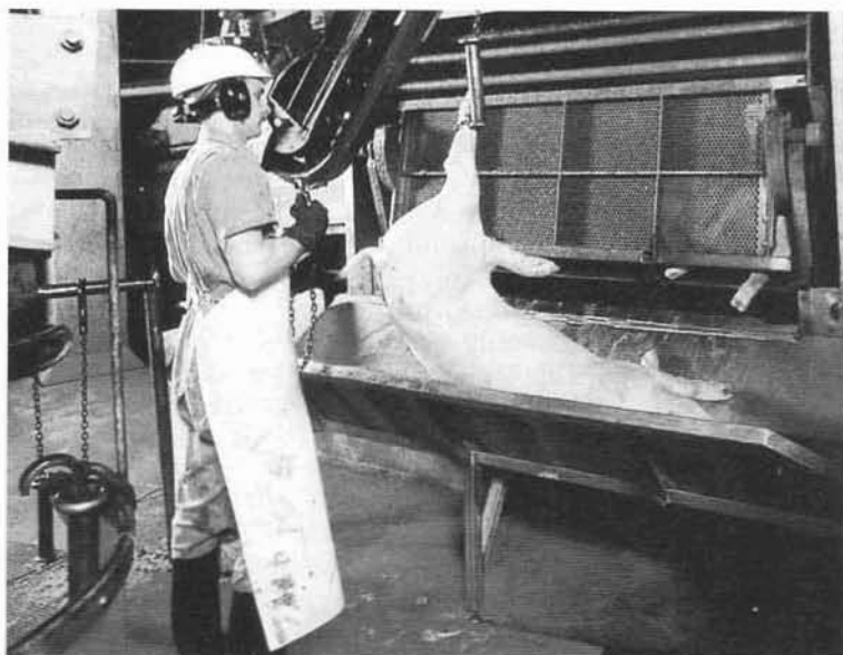
Fig. 8.4 CO 2 anaesthesia. Oval tunnel/Combi system showing convenient shackling position after stunning. (By courtesy of Messrs SFK Meat Processing A/S, Albuén 37, DK 6000, Kolding, Denmark)
