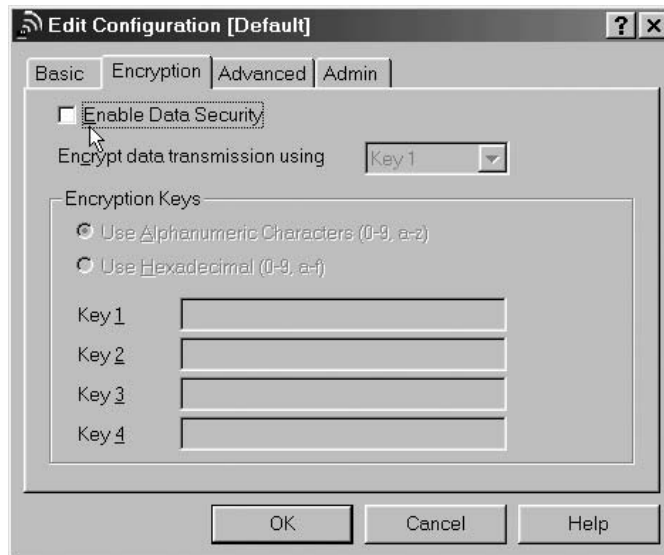
Figure 4.4 The Orinoco Encryption tab permits up to four keys to be configured for use. If not edited, the default of no encryption is used.
