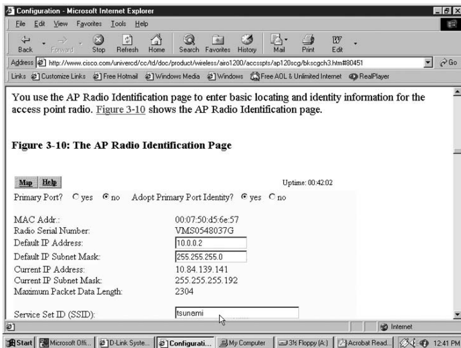
Figure 5.2 From the Cisco Web site you can view access point documentation that indicates the use of tsunami as the Service Set ID (SSID).
