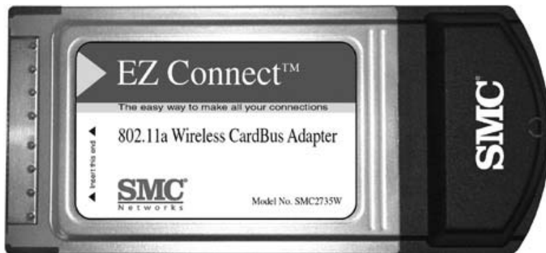
Figure 1.1 The SMC Networks 802.11a Wireless Card Bus Adapter (photograph courtesy of SMC Networks).
