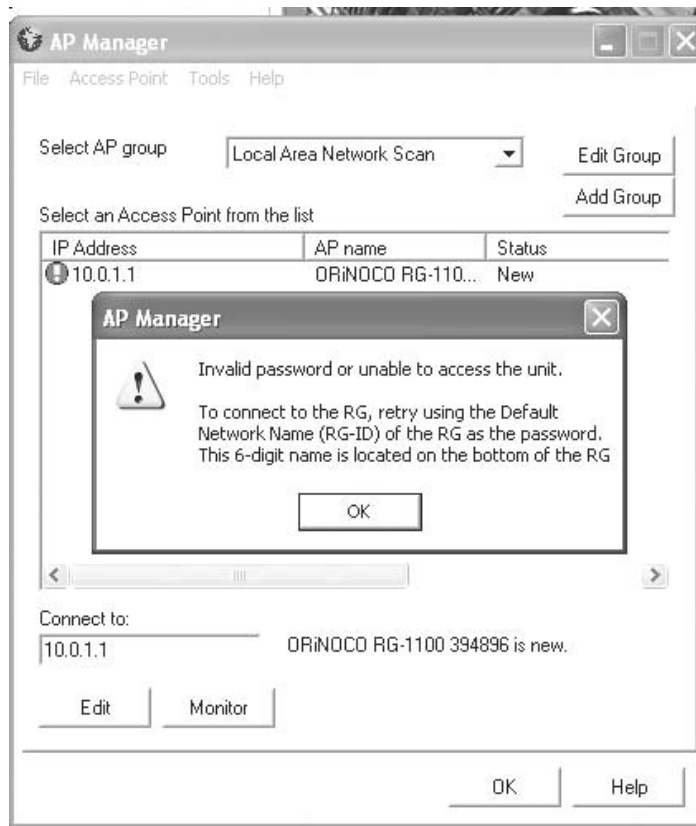
Figure 5.14 Although the Agere Systems' AP Manager indicates the 6-digit network name should be used to connect to a Residential Gateway, this author used the last 5 digits of the network name.
