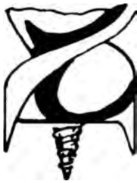
center bit showing cutting end
