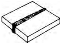
welded butt joint
