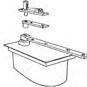
checking floor hinge
