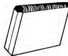
edge joint, 2 (welded)
