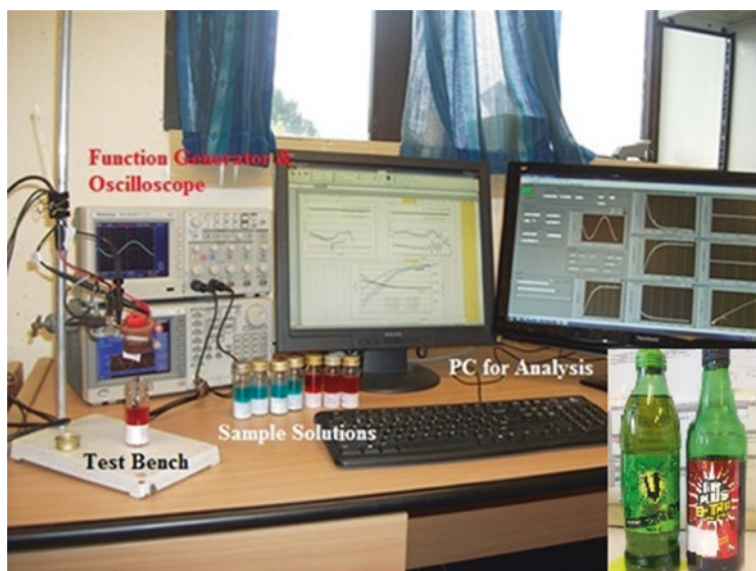
Fig. 5.12 Test bench setup for DEHP-spiked energy drinks
