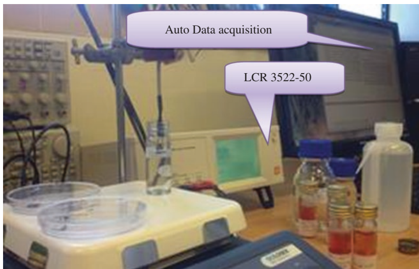
Fig. 4.3 Laboratory test bench for EIG testing
