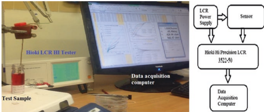
Fig. 2.10 Laboratory test bench with Hioki Hi Precision LCR and data acquisition system
