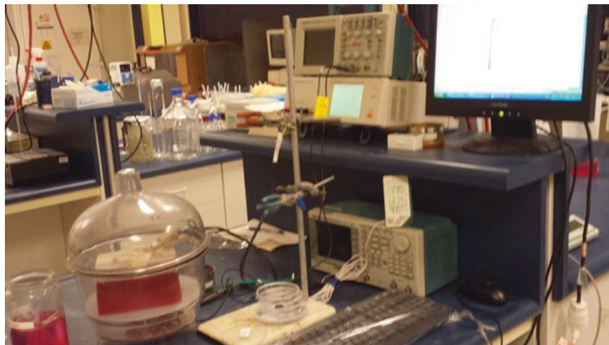
Fig. 6.12 Laboratory test bench setup for MIP coated sensor
